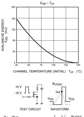
$EAS = \frac{1}{2} \cdot L \cdot l^2 \cdot$ BVDSS BVDSS - VDD  $R_G = 25 \Omega$  $V_{DD} = 90 V, L = 22.5 mH$
